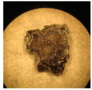
Microscope view of a sample of FeS, a common material found in iron meteorites. This sample will be used for high temperature experiments of mobility of Lead (Pb), which is a product of radioactive decay or Uranium and used to measure the ages of iron meteorites. Image courtesy of Dr. Heather Watson.
